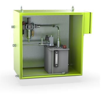
To operate the Compactus it should be supplied with pneumatic pressure and electrical control voltage. With the ratio of 1:44, approximately 200 bar hydraulic pressure can be achieved with only 4,5 bar pneumatic pressure.
