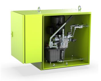
**DH 2400:** Unit with "Double control valves" for critical applications such as overhead cranes, etc. Other options are an accumulator, hand pump, pressure switches and additional filter unit.
