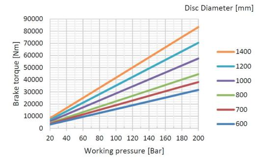
The braking torque is calculated from the following formula:
