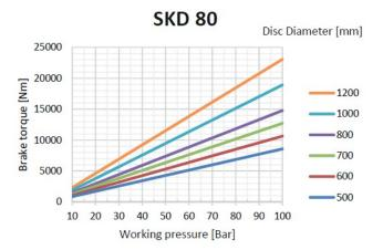
The braking torque is calculated from the following formula:
